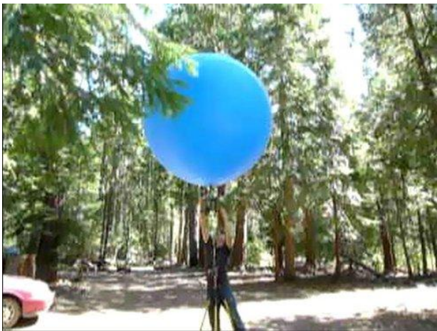
6ft cloudbuster balloon. Lift is 7lbs when slightly overinflated to 6ft. Rated diameter is 5.5ft
